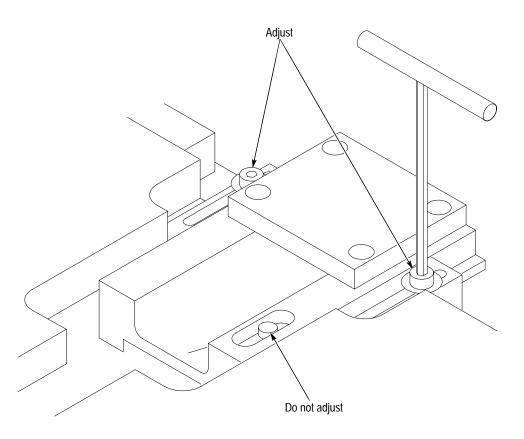
Figure 6–1: Bar code scanner adjustment screws
