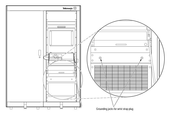
Figure 7–1: Wrist strap grounding connections
