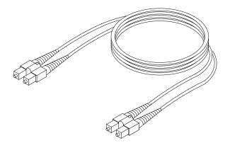
Figure 7–3: Duplex fiber optic cables
