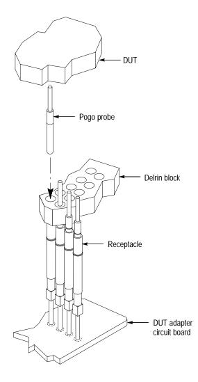
Figure 7–7: Through-hole Pogo probe replacement
