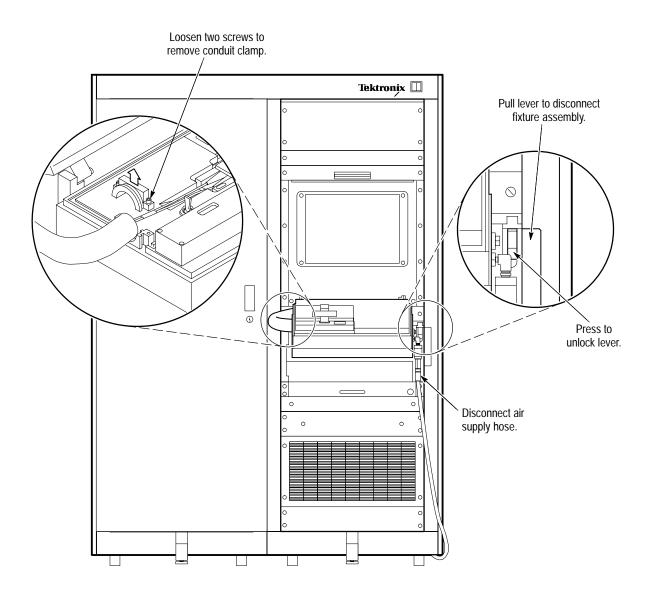
Figure 7-4: Test fixture removal
